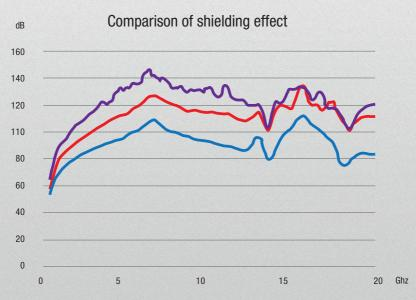
Shielding effectiveness measured using Nolato cavity to cavity test method
