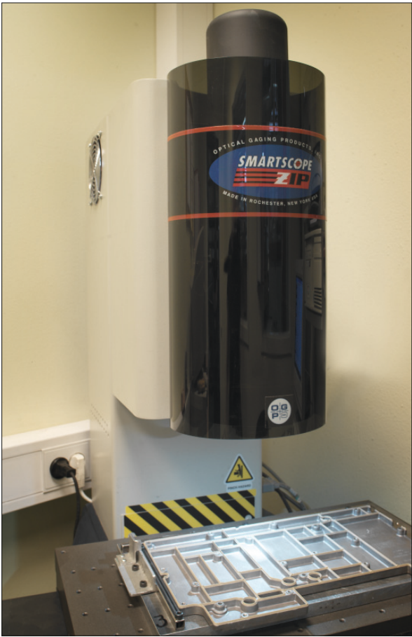
Picture 16. An optical measuring machine could be used for height and width measurement
