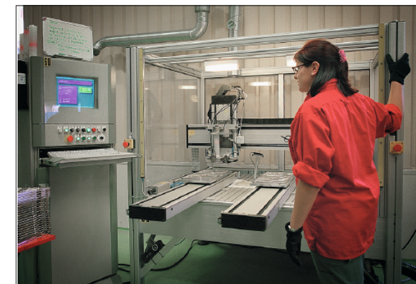
Picture 7. Example of a manually feed dispensing unit.
