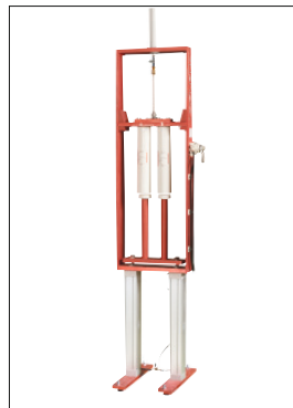
Picture 6. The fixed ratio static mixer from Nolato.
