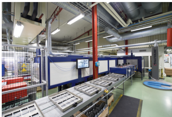
Picture 11. Example of hot air conveyor oven with forced ventilation.
