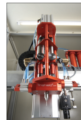
Picture 9. Example of a Trishield Soft® dispensing head.
