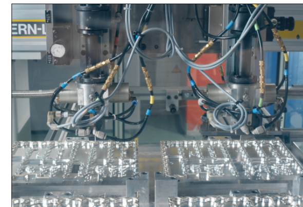
Picture 8. Example of an automated production cell with two head dispensing.
