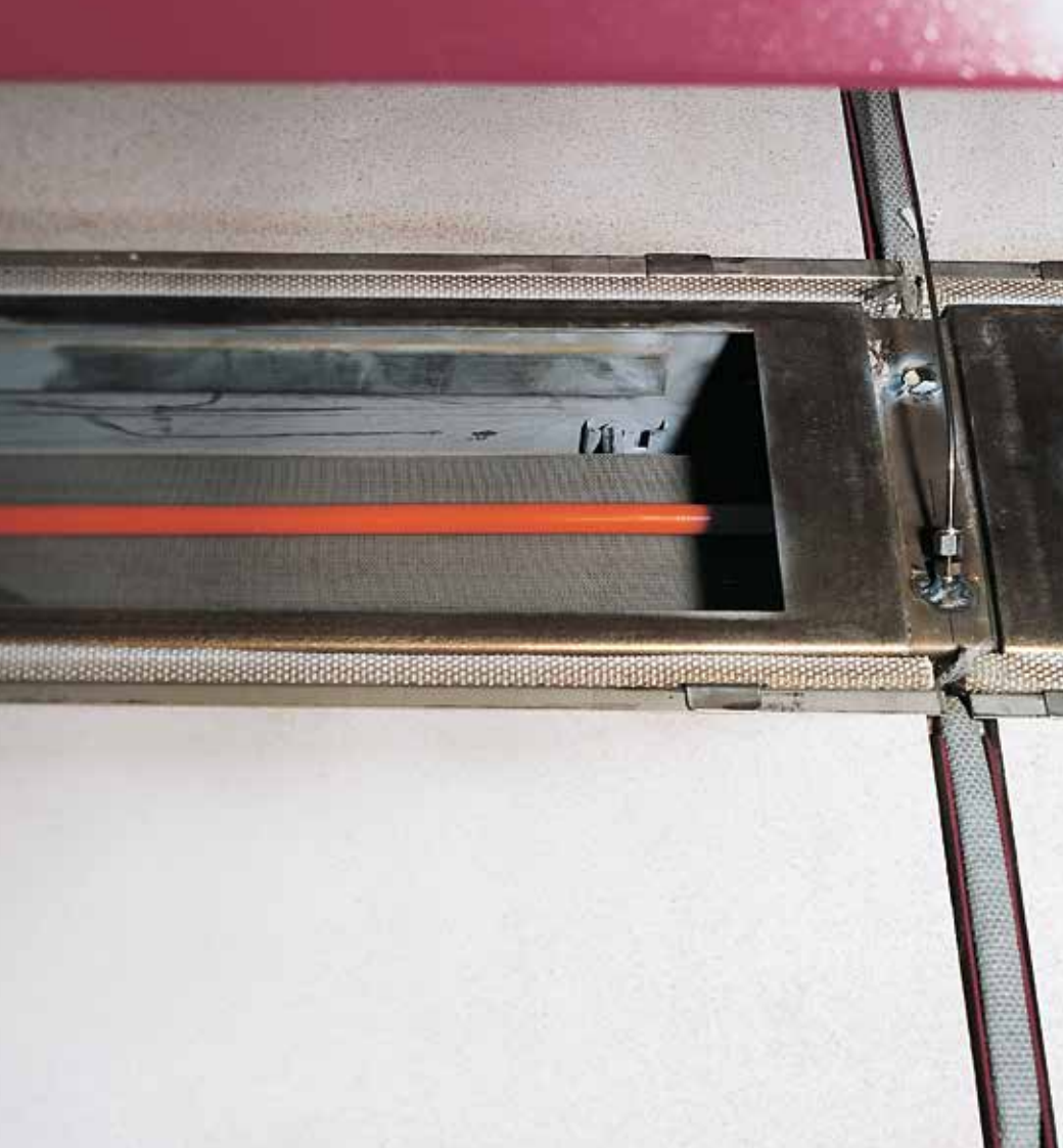
Hose vulcanization in a horizontal hot-air tunnel
