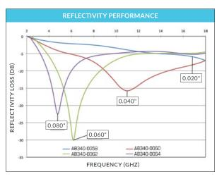
ELECTRICAL PERFORMANCE: The performance plot shown below illustrates the reflection loss performance of this material. Reflection loss is measured on a NRL arch, for more information on the NRL arch test set-up, please contact a Modus technical representative. Additional electrical test data may be available upon request.
