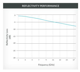
The performance plot sho on the left, illustrates the reflection loss performance of this material. Reflection loss is measured on a NRL arch. For more information on the NRL arch test set-up, please contact a Modus™ technica representative. Additional electrical test data may be available upon request
