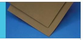
HiMag<sup>™</sup> Cavity Resonance Absorber die-cut parts and gaskets are thin, magnetically loaded sheet stock, having high loss at microwave frequencies, while maintaining the desirable characteristics of elastomeric binders. Cavity Resonance Absorbers are designed to exhibit high loss and are intended to be applied to metal surfaces inside microwave cavities to reduce the Q of the cavity.
