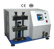
Fully-compliant A-A-59588, Class 3B silicones must pass the DeMattia Flex Resistance Test, a dynamic test that measures crack growth in inches over thousands of flexural cycles. The ASTM D813 - 07(2014) Standard Test Method for Rubber Deterioration-Crack Growth defines this testing protocol.
