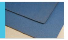
WesShield™ EMI shielding materials have been specifically designed to be used in the most demanding military and commercial applications. WesShield™ RC350-2170 is a high performance 65 durometer EMI shielding silicone compound that is filled with silver-plated aluminum particles.
