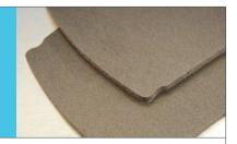
WesShield™ EMI shielding materials have been specifically designed to be used in the most demanding military and commercial applications. WesShield™ RC350-2210 is a high performance 60 durometer EMI shielding graphite filled flame retardant silicone compound that is nickel coated.
